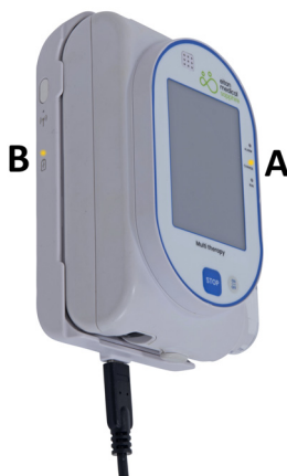
Figure 2.29. Recharge de la pompe Sapphire via le Sapphire Connect
